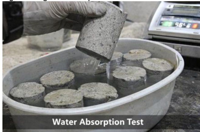
Figure 6 Water absorption test
