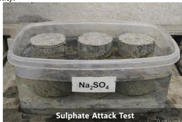
Figure 10 Sulphate attack test
