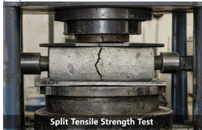
Figure 4 Split tensile test
