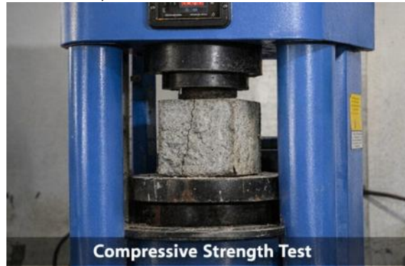
Figure 3 Compressive strength test
